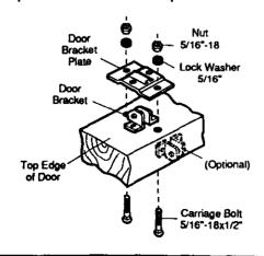
NOTE: The door bracket may be installed on face of door if required for your installation. (Refer to dotted line drawing.) HOWEVER, drill 3/16" pilot holes and substitute 5/16" × 1-1/2" lag screws (not supplied) to fasten the bracket to the door.
